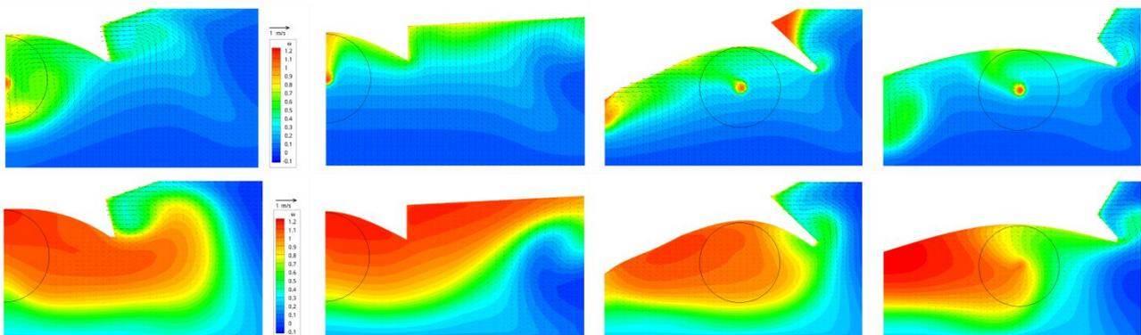
Figure 6 – Computed wake fields of the four models M2051 to M2054 (left to right). Top row for water depth  $h=7.50$  m and bottom row for  $h=3.50$  m.
