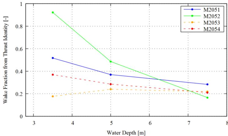
Figure 4 – Wake fractions based on thrust identity for all four models and three water depths.
