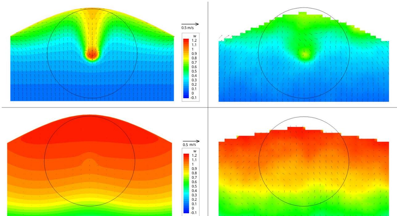
Figure 5 – Comparison of computed (left) and measured (right) wake fields for M2052. Top row at  $h=7.50$  m and bottom for  $h=3.50$  m water depth.
