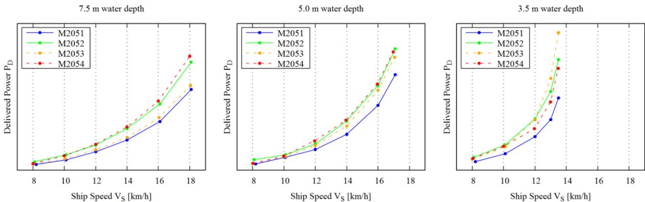
Figure 3 - Delivered power vs. velocity. Comparison of all vessels at 7.5 m (left), 5.0 m (middle) and 3.5 m (right) water depth
