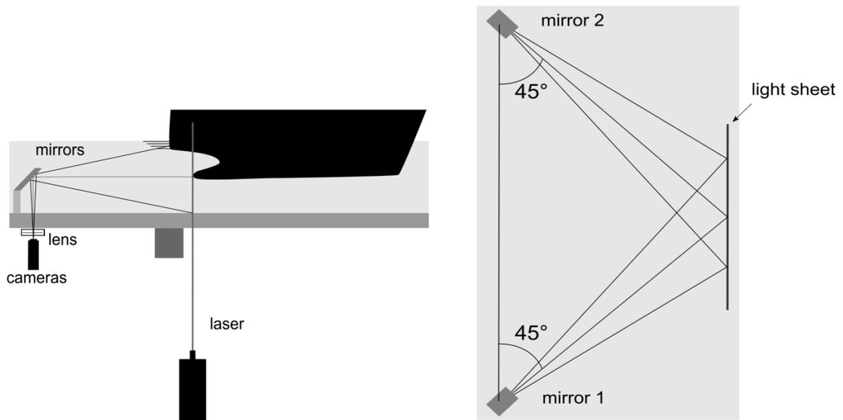
Figure 1 - PIV Setup. (left) side view. (right) top view
