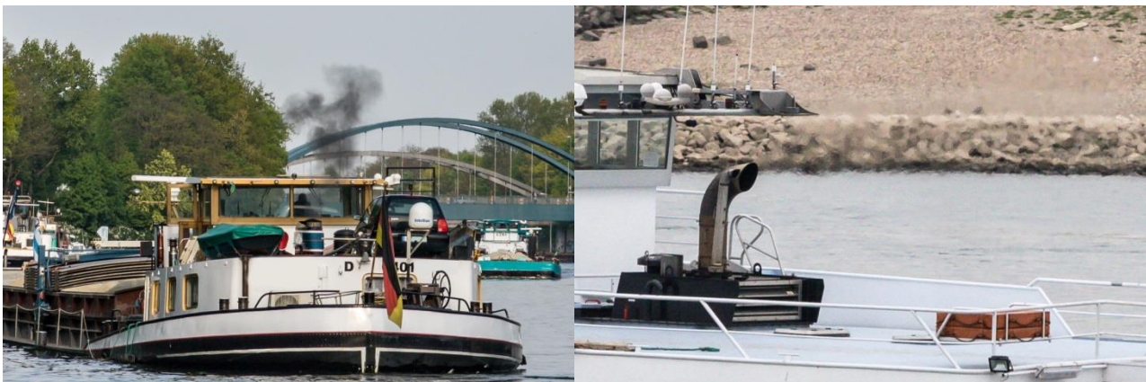
Figure 2: Pictures of exhaust plumes (left: engine reversing, right: typical appearance at steady state operation)
