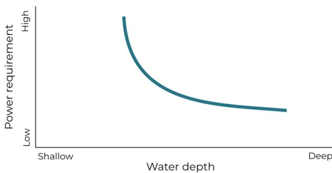
The relationships between required power, velocity of the ship and water depth are the main basis for EEN. This principle can be used to reduce energy consumption. The three most important facts are:
