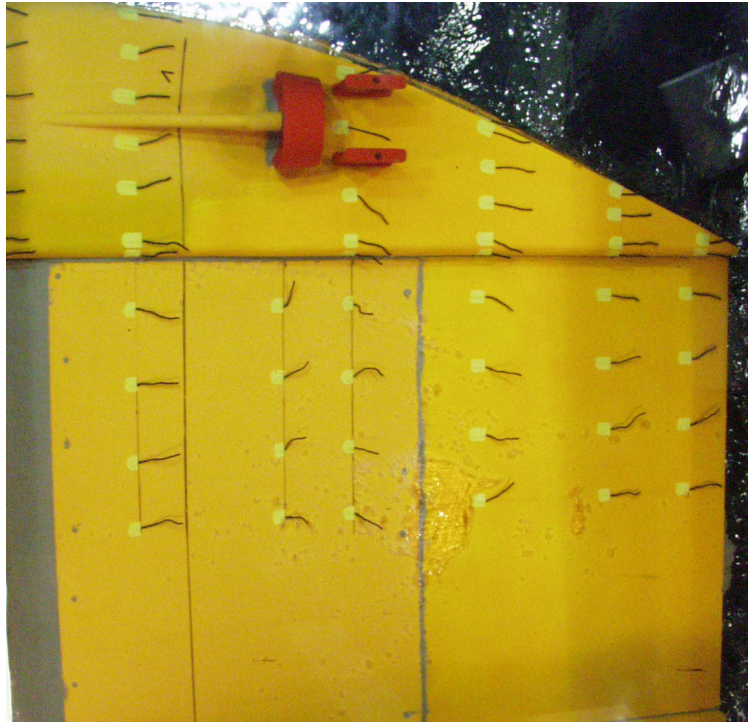
Rheinschiff, Formvariante 7, Propulsion, V = 14,0 \text{ km/h} , (Vers.-Nr. 067-02-01)
