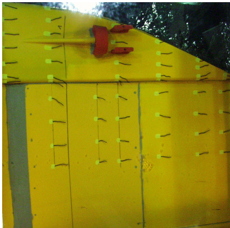
Rheinschiff, Formvariante 7, Widerstand, V = 14,0 \text{ km/h} , (Vers.-Nr. 068-02-03)
