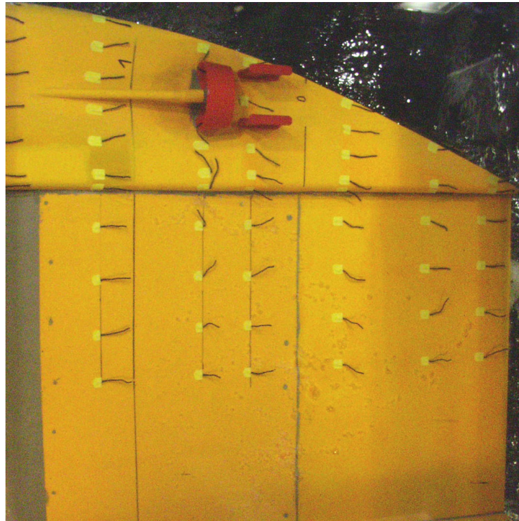
Rheinschiff, Formvariante 8, Propulsion, V = 14,0 km/h, (Vers.-Nr. 089-02-05)
